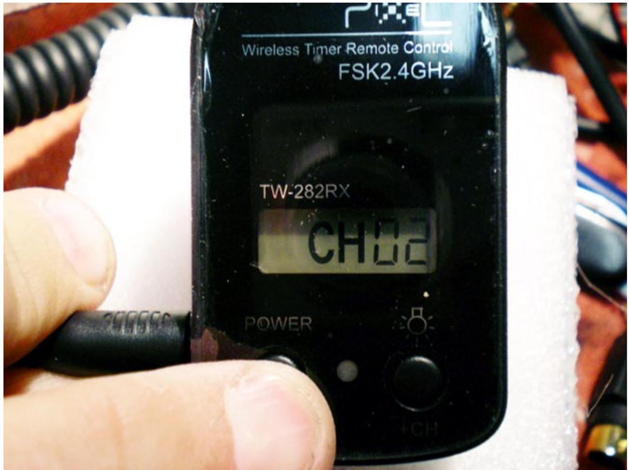
Next, take the wireless hand controller and press any buttons to turn it on. The hand controller will show a channel on the display as shown below
