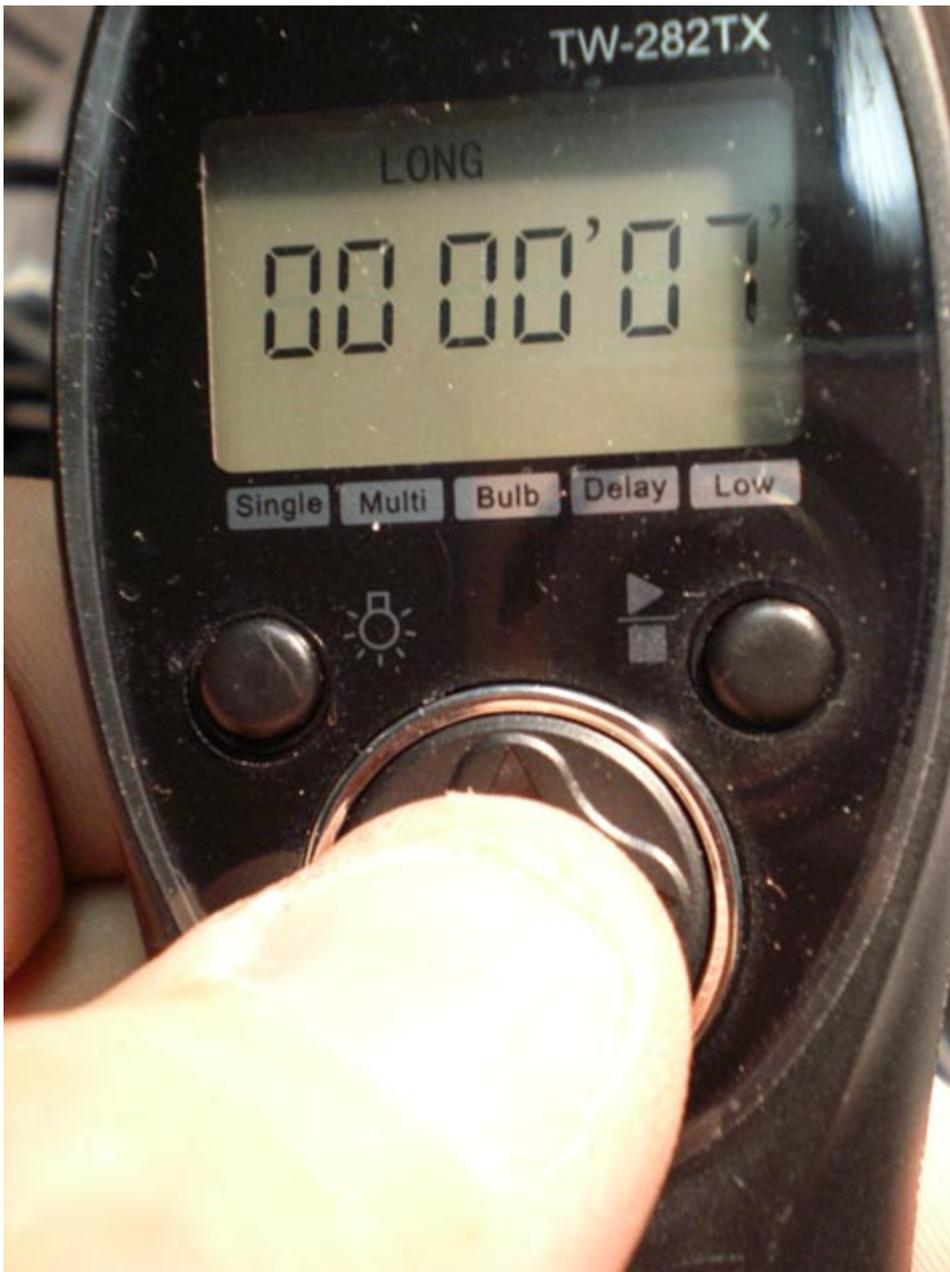
To activate the camera into 7 seconds integration with AUTO REFRESH, simply hit the upper right button which activate or stop the countdown as shown in picture below. Note the picture showing countdown to 2 seconds and will start over automatically to 7 seconds once the image has been taken and transferred to monitor.
