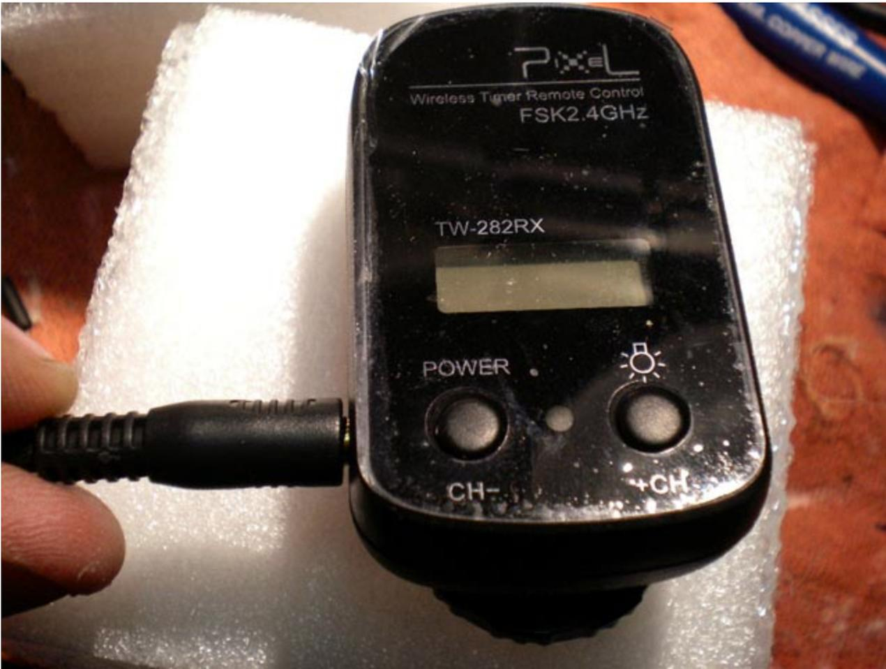
Next, turn on receiver by holding the left button called POWER for 3 to 4 seconds. The display will show either a blank channel or a channel number as shown in the picture below. You can change channel by pressing both buttons at the same time for 3 to 4 seconds until display flashes. Then select the channel of your choice.
