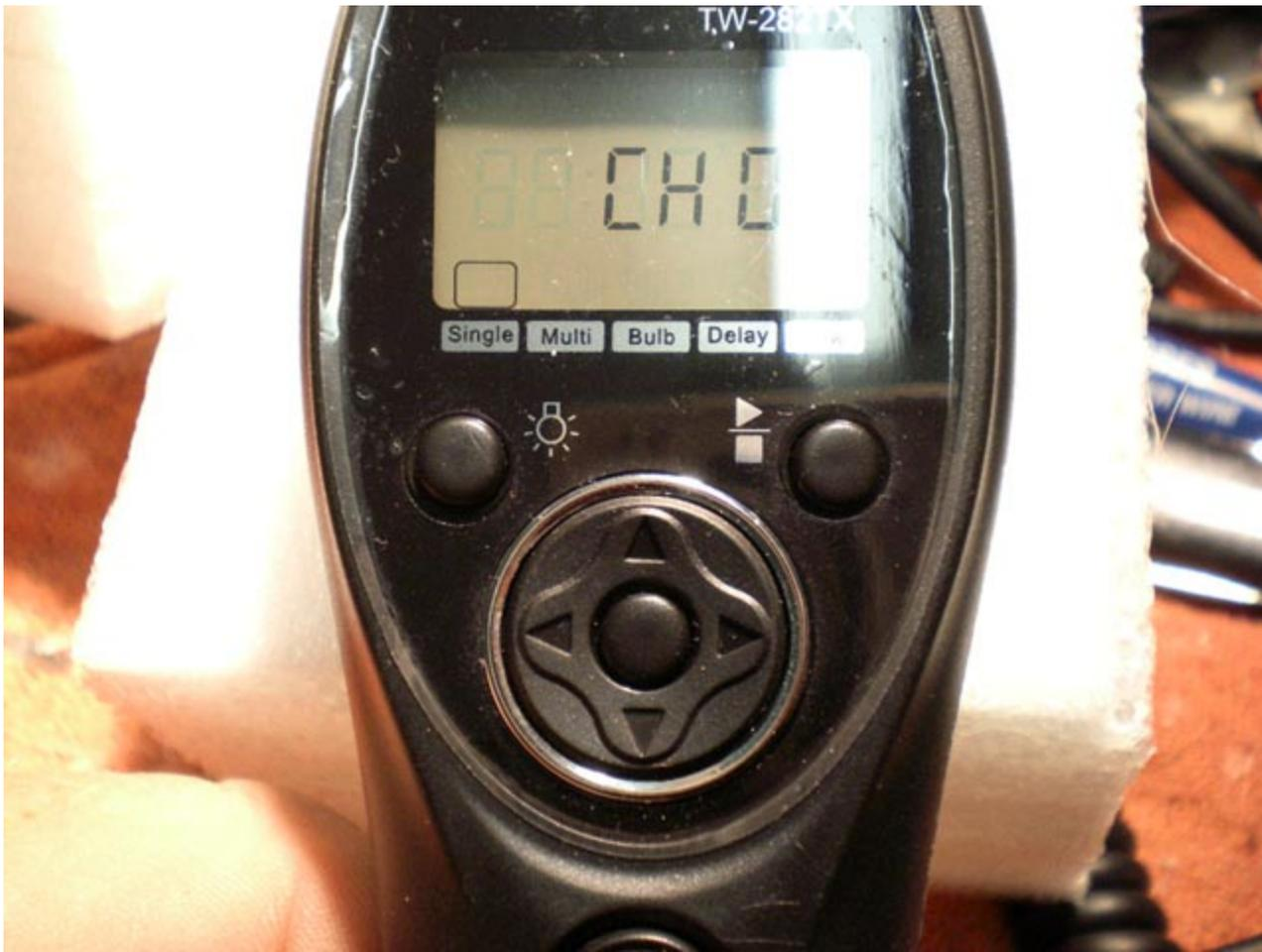
Next, Press the left or right arrows to select CH in the upper display. Press center key located between the arrows until display flashes. Next select the channel number to match the receiver channel by pressing the up or down arrow. Press center key to lock the channel.
