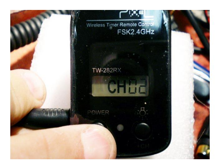
Next, take the wireless hand controller and press any buttons to turn it on. The hand controller will show a channel on the display as shown below
