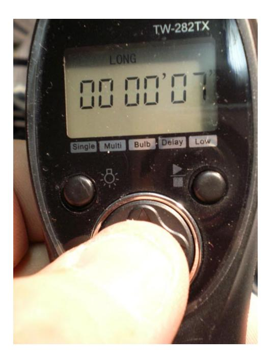
To active the camera into 7 seconds integration with AUTO REFRESH, simply hit the upper right button which activate or stop the countdown as shown in picture below. Note the picture showing countdown to 2 seconds and will start over automatically to 7 seconds once the image has been taken and transferred to monitor.
