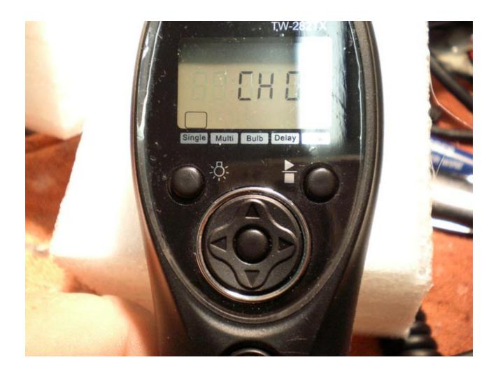
Next, Press the left or right arrows to select CH in the upper display. Press center key located between the rarrows until display flashes. Next select the channel number to match the receiver channel by pressing the up or down arrow. Press center key to lock the channel.
