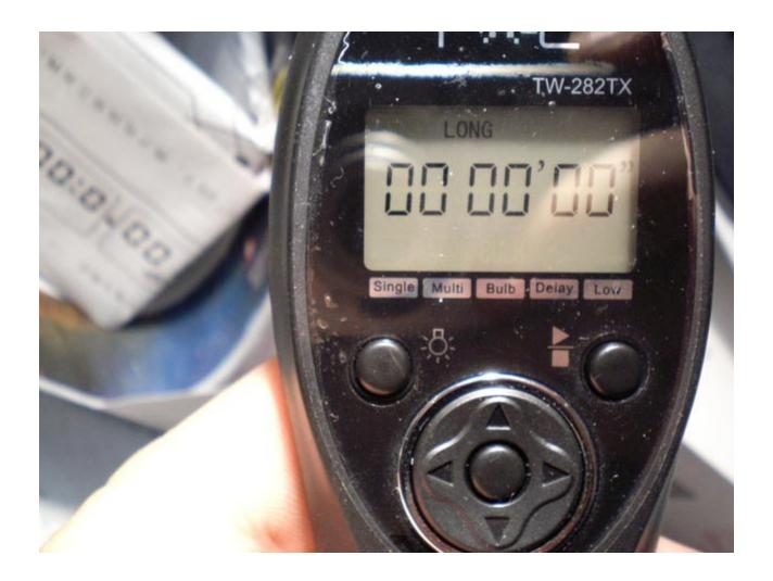
Next, press the right or left arrow until upper display indicate LONG as indicated by the picture above. This is where the integration time is entered. For this example, we will use 7 seconds integration
