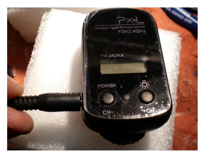
Next, turn on receiver by holding the left button called POWER for 3 to 4 seconds. The display will show either a blank channel or a channel number as shown in the picture below. You can change channel by pressing both buttons at the same time for 3 to 4 seconds until display flashes. Then select the channel of your choice.
