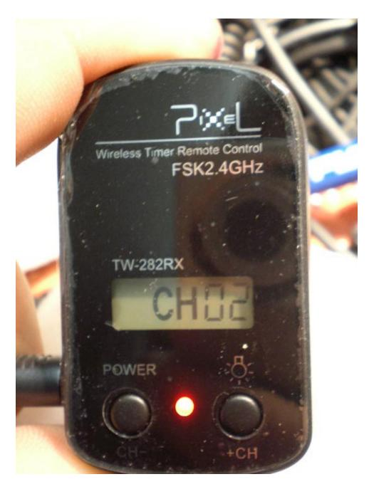
After the observing / imaging session, please remember to turn OFF the Receiver by pressing POWER for 4 seconds or until display goes blank. The hand controller will automatically shut down by itself in one minute. A light can be turned on momentarily by pressing the upper left button for 4 seconds or until display light comes on. It will turn off automatically after 6 seconds or more to save battery power. For long term storage, remove batteries from hand controller and receiver.
