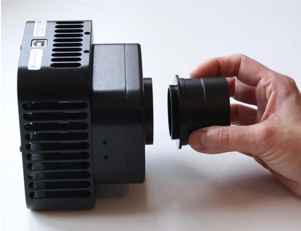
**NOTE:** There are three small set screws in the mounting collar of the camera body. Make sure these are out far enough to allow the nosepiece to fully seat. After the nosepiece is installed, you can either tighten these down for increased security or permanent installations, or remove them. The use of these screws is optional.
