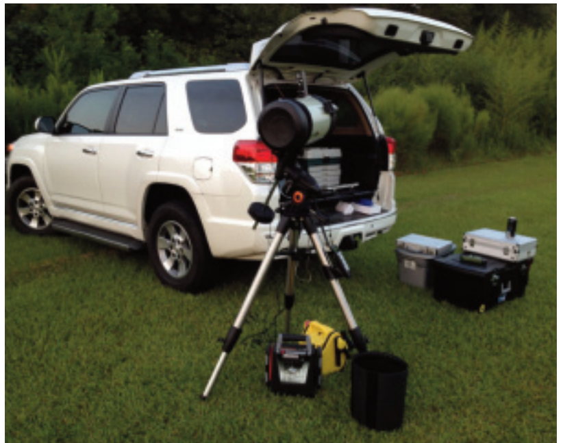
Image 4 - For the purposes of this article, Uncle Rod tested the MallinCam Junior Pro with his Celestron Edge 800 SCT and VX German equatorial mount.
